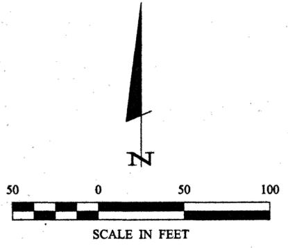
ORIENTATION OF THIS BEARING SYSTEM IS BASED ON THE EAST LINE OF THE LOT 7 TO HAVE AN ASSUMED BEARING OF N 0° 41' 30" E.
