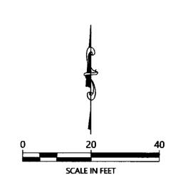
ORIENTATION OF THIS BEARING SYSTEM IS BASED ON THE NORTH LINE OF BLOCK 22, ORIGINAL PLAT OF WALKER, TO HAVE AN ASSIGNED BEARING OF S 89°58'42"E.
