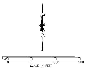
THE BEARING ORIENTATION OF THIS SURVEY IS BASE ON CASS COUNTY NORTH ZONE NAD(83)
