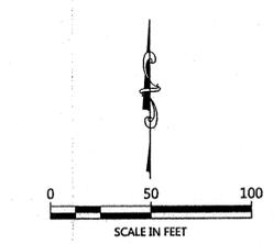
ORIENTATION OF THIS BEARING SYSTEM IS BASED ON THE EAST LINE OF LOT 1, GILLESPIE'S SUBDIVISION TO HAVE AN ASSIGNED BEARING OF N 00°01'03" E.
