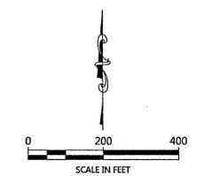
ORIENTATION OF THIS BEARING SYSTEM IS BASED ON THE NORTH-SOUTH QUARTER LINE OF SECTION 31 TO HAVE AN ASSIGNED BEARING OF N 00°54'40" E.
