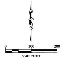
ORIENTATION OF THIS BEARING SYSTEM IS BASED ON THE SOUTH LINE OF GOVERNMENT LOT 4 TO HAVE AN ASSIGNED BEARING OF N 89°51'39" E.
