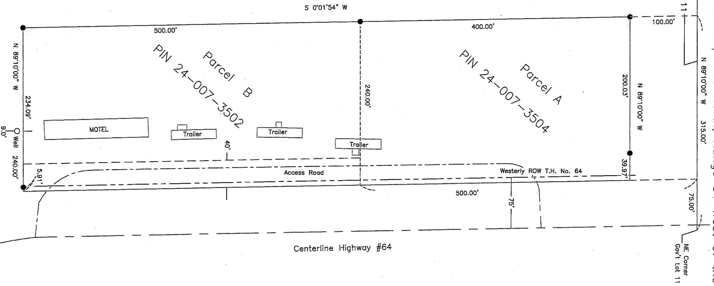
The North line of Gov't Lot 11 of Section 7 is assigned a bearing of N 89°10'00" W.
