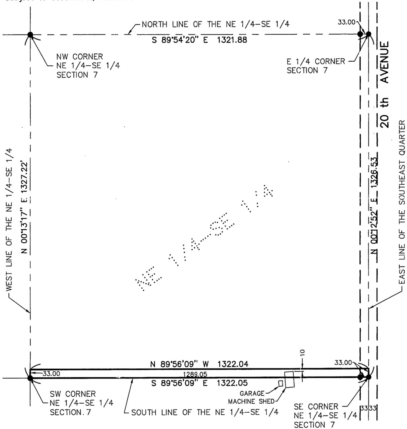
ORIENTATION OF THIS BEARING SYSTEM IS BASED ON THE SOUTH LINE OF THE NE 1/4-SE 1/4 TO HAVE AN ASSUMED BEARING OF S 89°56'09" E.
