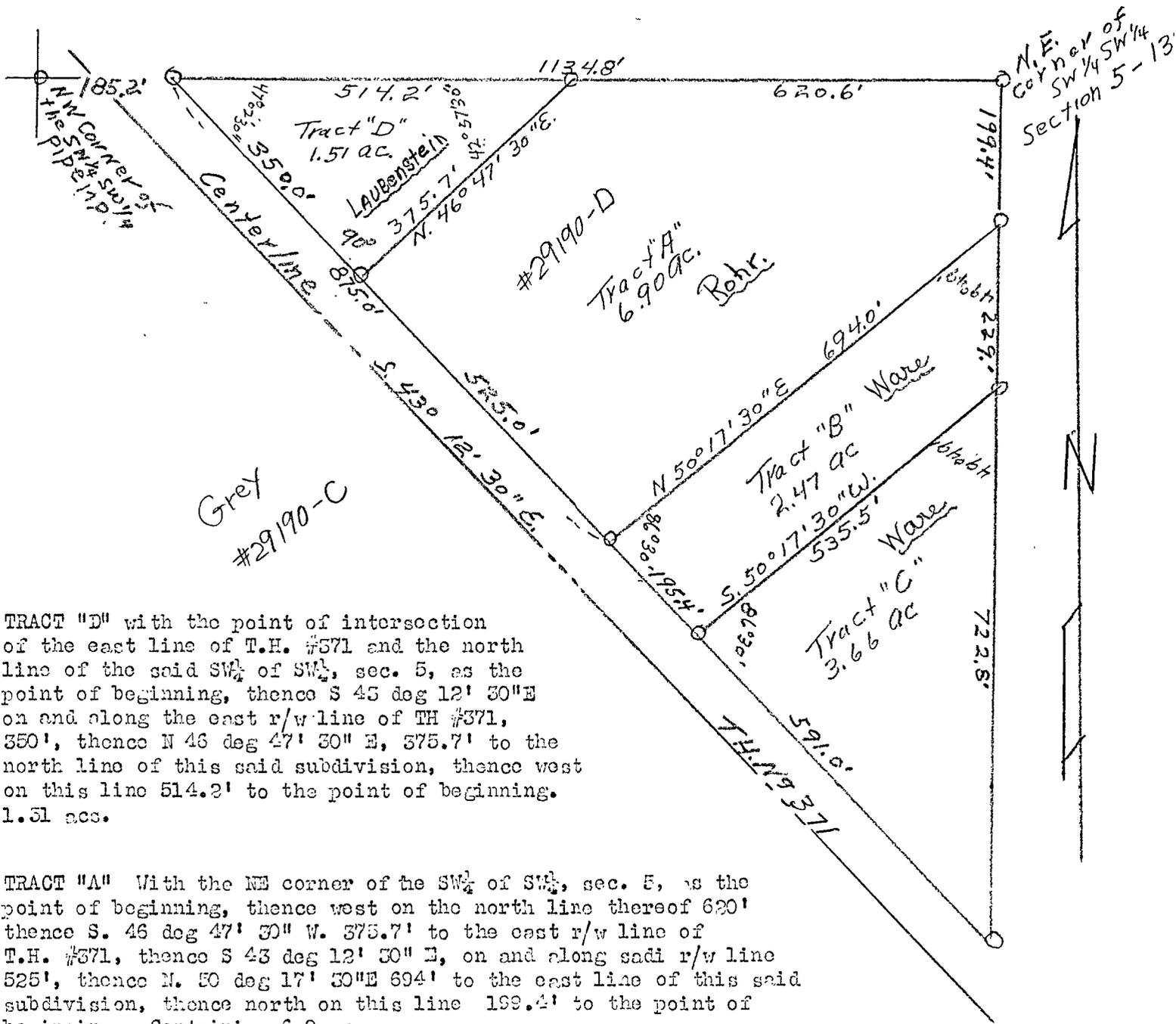
TRACT "D" with the point of intersection of the east line of T.H. #371 and the north line of the said SW<sup>1</sup>/<sub>4</sub> of SW<sup>1</sup>/<sub>4</sub>, sec. 5, as the point of beginning, thence S 45 deg 12' 30" E on and along the east r/w line of TH #371, 350', thence N 46 deg 47' 30" E, 375.7' to the north line of this said subdivision, thence west on this line 514.2' to the point of beginning. 1.51 acs.
