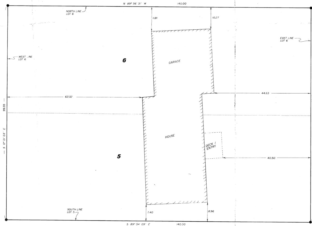
NOTE: OFFSET DIMENSIONS AS SHOWN ARE MEASURED TO THE BUILDING CORNERS. THERE IS A 1 FOOT EAVE OVERHANG AROUND ALL OF THE HOUSE AND GARAGE.
