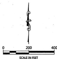
ORIENTATION OF THIS BEARING SYSTEM IS BASED ON THE NORTH LINE OF GOVERNMENT LOT 1, SECTION 32, T141N, R31W TO HAVE AN ASSIGNED BEARING OF N 88°30'39" E.
