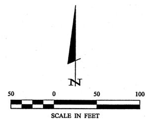
ORIENTATION OF THIS BEARING SYSTEM IS BASED ON THE SOUTH LINE OF GOVERNMENT LOT 1 TO HAVE AN ASSIGNED BEARING OF S 89°49'57" W.
