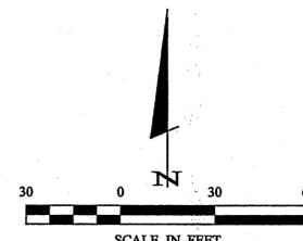
ORIENTATION OF THIS BEARING SYSTEM IS BASED ON THE SOUTH LINE OF THE SOUTHWEST QUARTER OF THE SOUTHEAST QUARTER TO HAVE AN ASSIGNED BEARING OF N 69°28'58" E.
