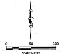
ORIENTATION OF THIS BEARING SYSTEM IS BASED ON THE SOUTH LINE OF LOT 72 TO HAVE AN ASSIGNED BEARING OF N 85°44'34" E.
