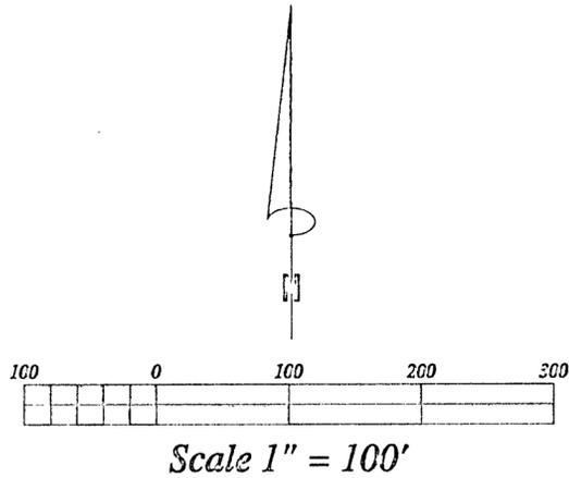
Orientation of this survey was based upon the south line of the Southwest Quarter of the Northeast Quarter, Section 7, T141N, R31W, which was assigned a bearing of S 72°10'30" W.
