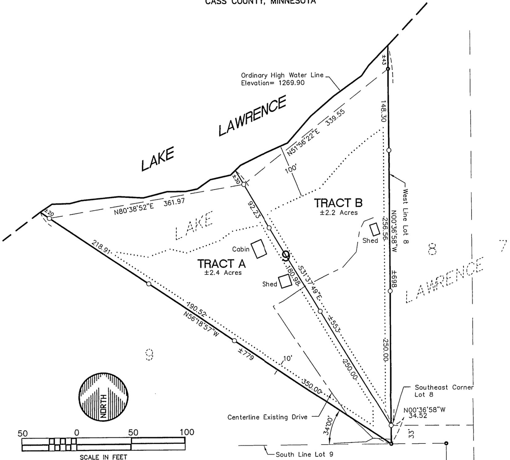
ORIENTATION OF THIS BEARING SYSTEM IS BASED ON AN ASSUMED DATUM
