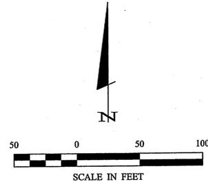
ORIENTATION OF THIS BEARING SYSTEM IS BASED ON THE NORTH LINE OF NORTHEAST QUARTER TO HAVE AN ASSUMED BEARING OF S 89° 49' 12" E.
