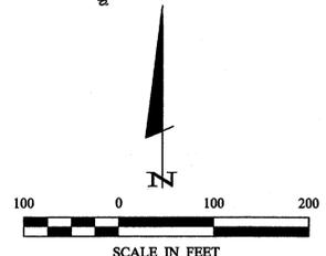
ORIENTATION OF THIS BEARING SYSTEM IS BASED ON THE NORTH LINE OF SECTION 9 TO HAVE AN ASSUMED BEARING OF N88°10'48"W.
