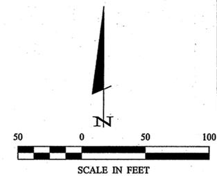
ORIENTATION OF THIS BEARING SYSTEM IS BASED ON THE WEST LINE OF GOVERNMENT LOT 1 TO HAVE AN ASSUMED BEARING OF S 05°13'31" W.
