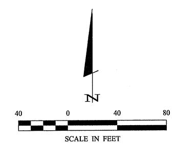
ORIENTATION OF THIS BEARING SYSTEM IS BASED ON THE WEST LINE OF GOVERNMENT LOT 1 TO HAVE AN ASSUMED BEARING OF S 01°16'50" E.
