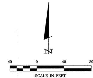
ORIENTATION OF THIS BEARING SYSTEM IS BASED ON THE NORTH LINE OF THE E 1/2 OF THE SW 1/4-SW 1/4 TO HAVE AN ASSUMED BEARING OF N 89°43'02" E.
