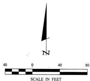
ORIENTATION OF THIS BEARING SYSTEM IS BASED ON THE SOUTH LINE OF GOVERNMENT LOT 7 TO HAVE AN ASSUMED BEARING OF N 89°50'42" W.
