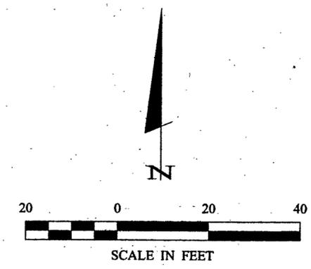
ORIENTATION OF THIS BEARING SYSTEM IS BASED ON THE SOUTH LINE OF LOT 2 TO HAVE AN ASSUMED BEARING OF S 89° 41' 11" W.
