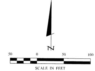
ORIENTATION OF THIS BEARING SYSTEM IS BASED ON THE NORTH LINE OF THE SW 1/4 - NE 1/4 TO HAVE AN ASSUMED BEARING OF N 86°09'43" E.
