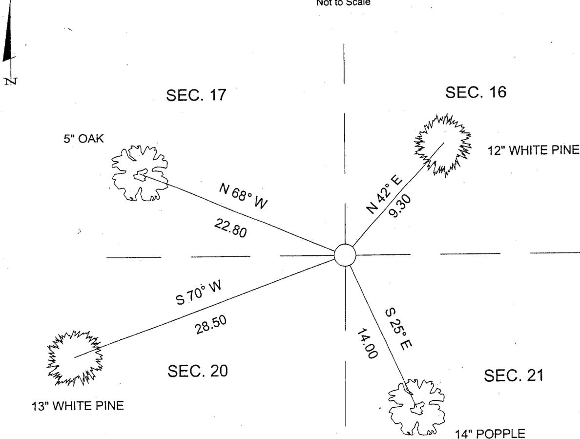
THE BEARING TREES WERE MARKED WITH BT TAGS AND NAILS AT BASE.
