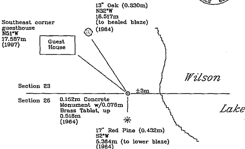
New bearing trees were blazed, scribed & painted red. A tag stating the bearing & distance was affixed to the tree. A nail was placed in the base of the tree and the distance was measured from the monument to the nail.
