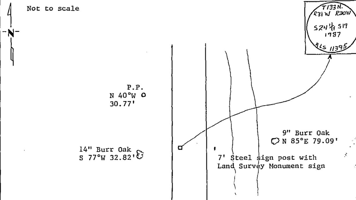
Trees double blazed, scribed, painted blaze orange and 54-3 Bearing Tree tag attached. Measurement taken to nail in side of tree.
