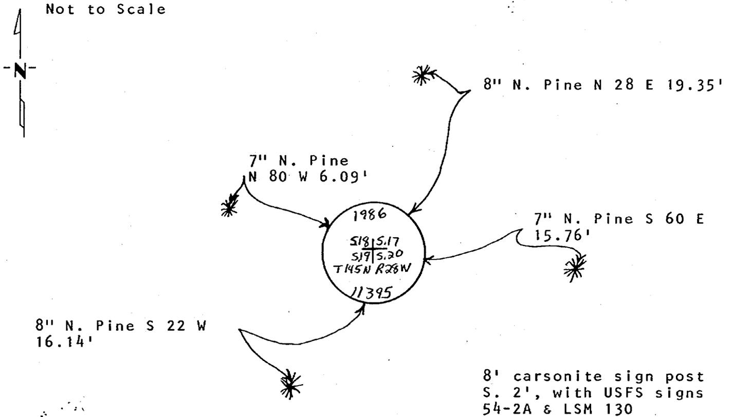
All measurements are to spks. in side of tree, trees are double blazed, scribed and painted red, with USFS 54-3 bearing tree tags attached.
