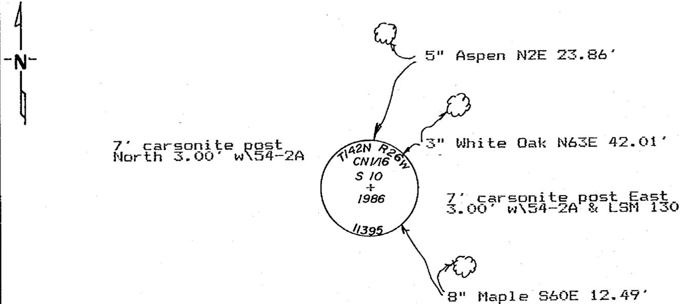
All measurements are to spks. in side of the tree, trees are double blazed and scribed and painted red with USFS 54-3 bearing tree tag.
