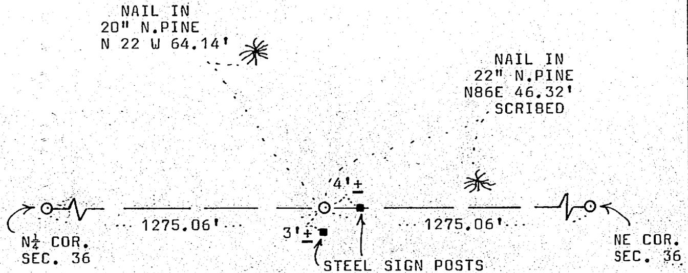
A 2" x 60" GALVANIZED IRON PIPE WITH A 3" MARKED BRASS CAP WAS SET FOR THE CORNER ON LINE AND MIDWAY BETWEEN THE NORTH QUARTER CORNER AND THE NORTHEAST CORNER OF SECTION 36.
