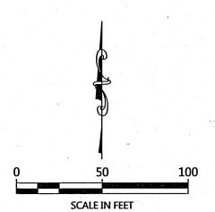
ORIENTATION OF THIS BEARING SYSTEM IS BASED ON THE EAST LINE OF GOVERNMENT LOT 4 TO HAVE AN ASSIGNED BEARING OF N 00°36'31" W.
