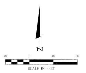
ORIENTATION OF THIS BEARING SYSTEM IS BASED ON THE NORTHERLY LINE OF LOT 6, BLOCK 8, INTERLACHEN LODGE TO HAVE AN ASSUMED BEARING OF S 54°05'50" E.
